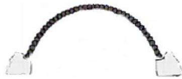
Step 1: Soilcrete jet grouting of the tunnel top heading.
