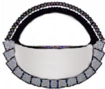
Step 3: Soilcrete jet grouting of the sealing base slab.
